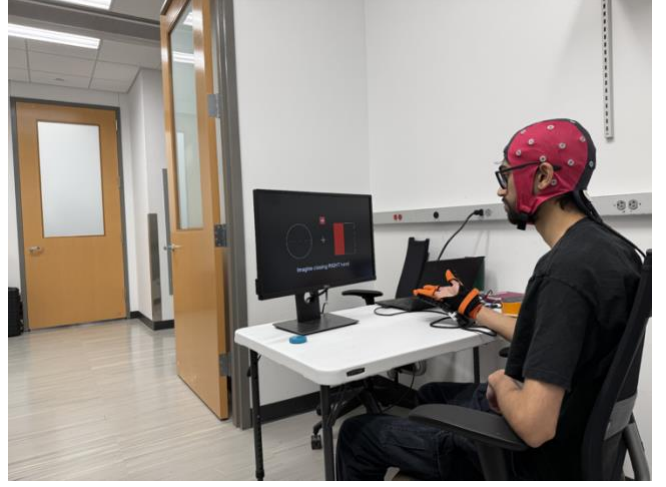
Fig. 1. Participant wearing 32-ch EEG cap with orthotic glove and FES, performing Online MI task.
